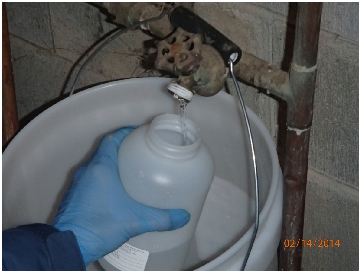
Photograph 3: Up close view of CESCO, Inc. collecting a sample directly from the spigot in the basement of Mary and David Cooper's residence on parcel # 220000047000, at 20411 Cadiz Road, Freeport, Ohio 43973.
