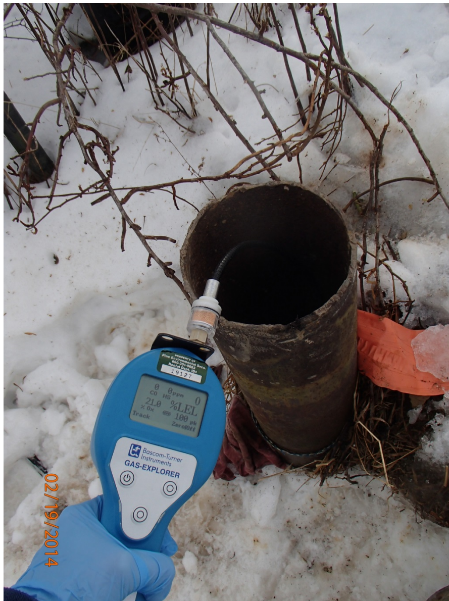
Photograph 2: Up close view of a Bascom-Turner Gas Explorer used to measure gases in the headspace immediately after the well cap is removed. The well is used to supply approximately 500 head of cattle on parcel # 220000226000, at 20633 Halfpenny Lane, Freeport, Ohio 43973.
